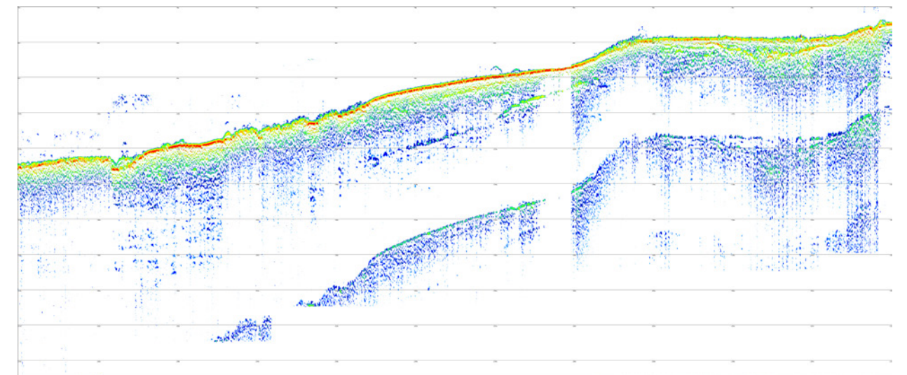
Fig. 21 Profile 20181123-121132, recorded by sub-bottom profiler (GEOmar Ltd.)
